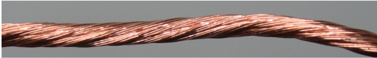
Close-up of the conductor rope
